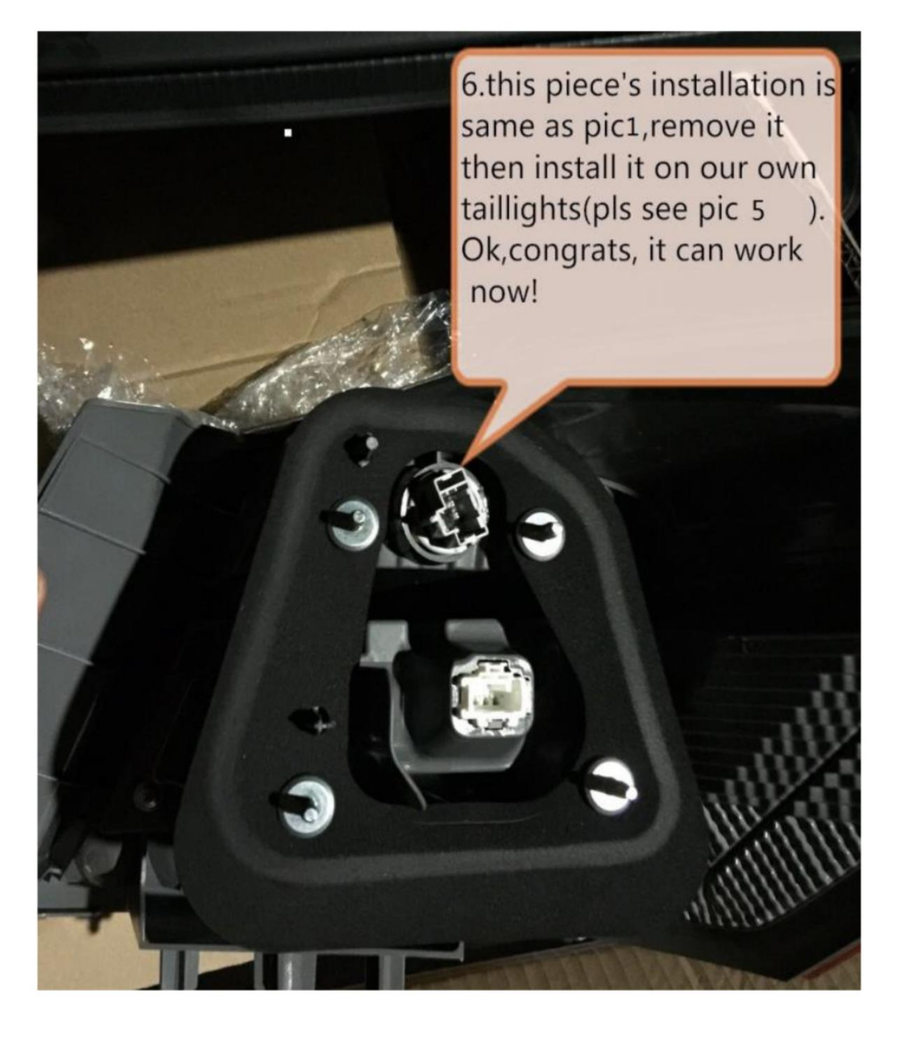
6.this piece's installation is same as step1, remove the socket then install it on our taillights' turning light wire.(see step 5)
