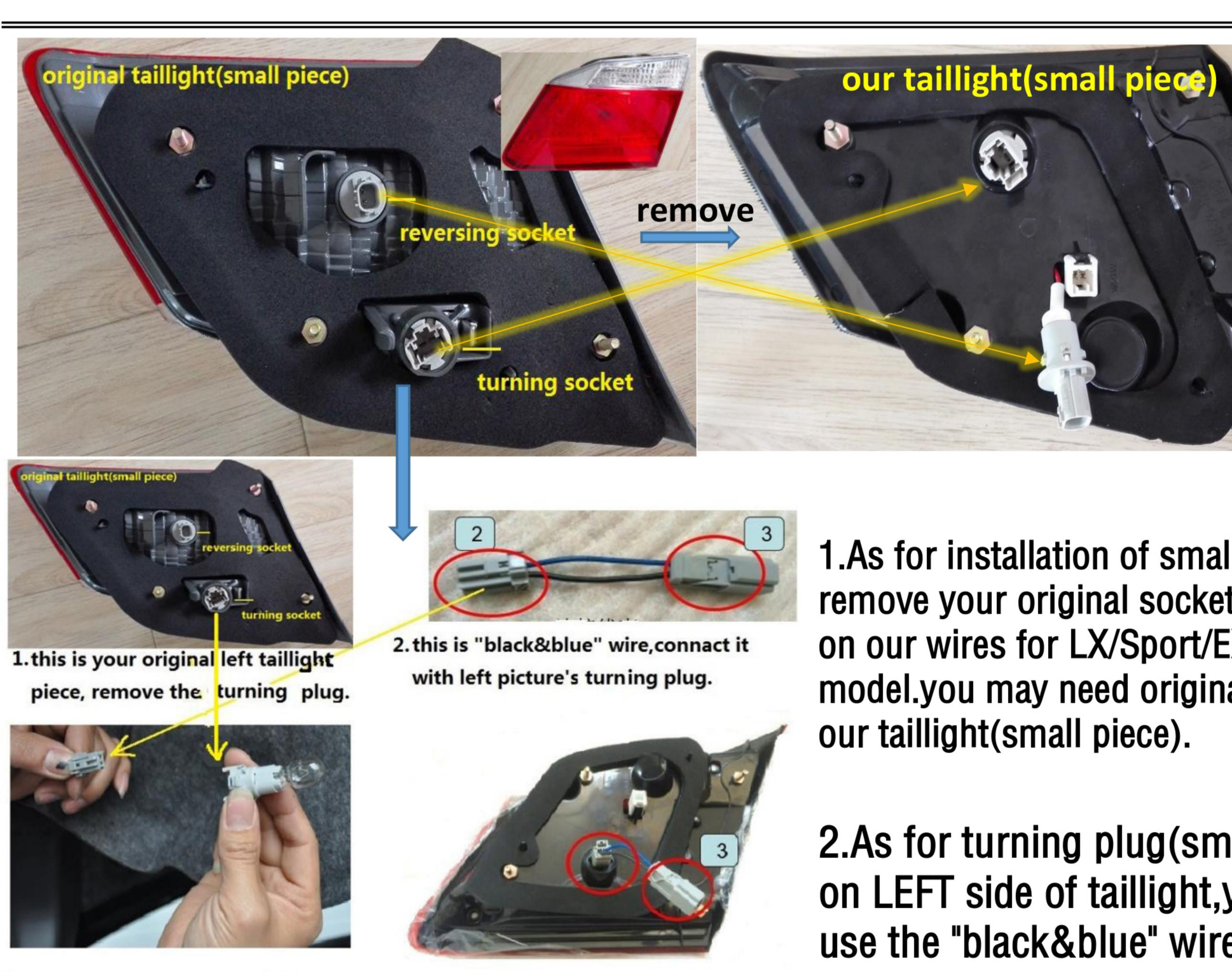
3.connect the plug and the wire 4. install this wire on our LEFT side taillight
